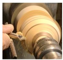
Mikeal laid out the lines where certain diameters and cuts would be made first. Then turning began with the champfers turned into the piece first.
