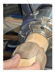
After initial turning, Mel retightened the turning in the chuck. You can see from the picture at left where the shape is beginning to appear.
