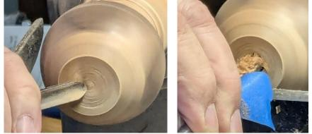
Using a "custom" blowpipe (*actually the barrel of a used Bic*<sup>TM</sup> *ballpoint pen*) Mel removed the shavings
