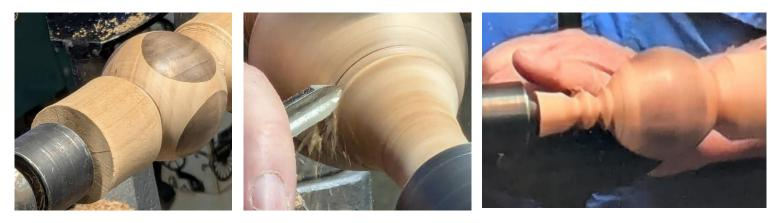
From left to right, the tailstock piece is reattached, the forming of the lower finial begins and the shape appears at right. Note there IS a line where the attachment was done. Not to worry, however, it will go away later.
