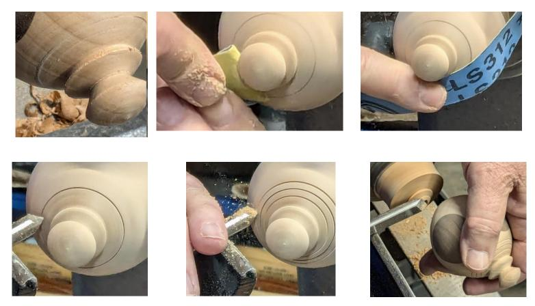
The joint line that indicated where the tailstock piece was rejoined is now the basis for some decorative cuts using the bowl gouge to score small lines and widen SLIGHTLY the original joint line. Once this is completed with some more LIGHT sanding, the ball is parted off. Note there appears to be a hole in the remaining piece in the headstock chuck. This would be used to attach a top finial which would then get the tree hanging wire.
