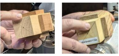
Mel's base piece on the right was made from Yellowheart which is a somewhat softer wood than the Cherry or Oak which would be glued on the outside. Mel stated that a firm, but softer wood is a little harder to turn once the hollowing begins but provides a better job when completed and is a little lighter in weight on the tree.
