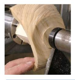
All that remains is to turn the tenon off on the bottom of the dish. A block holds the dish on the chuck side and the tailstock is used to hold the piece to turn the tenon off. This completes the soap dish and with some minor hand sanding on the edges that could not be done turning on the lathe, applying some kind of penetrating finish that is not toxic, the dish is ready to use,.
