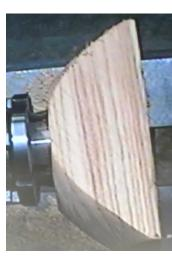
Block thickness can be seen at left for the external shape being turned. This is necessary to provide the depth on the finished turning to hold the soap bar.
