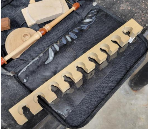
Tool Holder fixture for lathe tools either in a tool panel or at the lathe.
