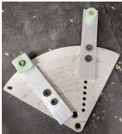
Steve Dougherty brought a couple of his jigs and fixtures he uses. The left hand one is a steady rest for long small, flexible turnings. The One at the right is ??.
