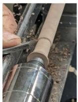
Continuing to form the shape of the pin and working a taper onto the turning which is rotating at about 1150-1500 RPM takes a careful feel and feed into the turning work.
