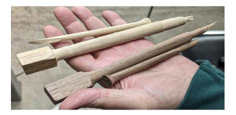
Danny also showed what can happen when the grain of the turning piece is not straight with the length of the blank. Turning seems to be doing fine and either the tool catches, a too-quick feed into the turning or a diagonal grain pattern allows the parts to separate.
