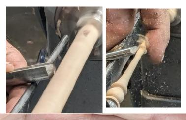
The part supported by the tail-stock will be removed on the finished pin as shown at left above.
