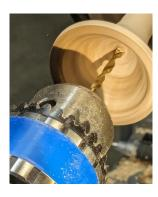
The diameter for fitting inside the body is turned and the base is hollowed out. Then using a large Cone Dead center (*actually live to turn*) the finished shape is turned on the outside of the insert. A hole is drilled to allow the salt to come out once the two parts are assembled together.
