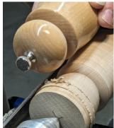
After changing chucks to an internal finger chuck and turning the blank around agein the "ball" or top of the shaker is begun. Comparing it to the pepper mill for spacing and size, the ball top is shaped.
