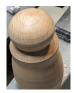
Using another blank about the same size as the original the insert that makes it into an "upside down" salt shaker is begun. It also sis made of Maple.
