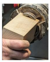
The blank is about 2-1/2" square and about 5" long. After locating the centr on both ends and marking, it the blank is inserted into a "One-Way" type 4-jaw chuck for turning.
