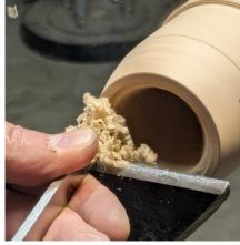
After finishing the shape of the outside a groove is turned into what will become the bottom to hold the shaker insert.
