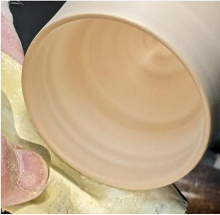
Note the smooth transition from side wall to bottom using the carbide insert tool as shown at the left. Once the basic shape is attained, the “boring” job of sanding takes place.
