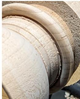
David used a ¼” ring tool to cut the ring loose on the underside of the ring from the main turning blank. At near left one can see the loose ring before removing extra stem material under it. The hardest part in ring turning now involves keeping the ring from interfering with material removal under the ring.
