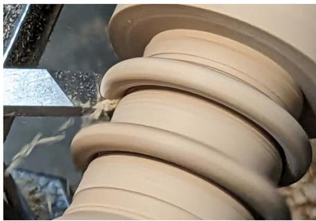
Upon “freeing” the second ring, some sanding is in order. Also, the stem needs to be thinned down to allow internal sanding of the rings. One trick David used was to attach the abrasive to the undeveloped stem and carefully hold the ring up to the abrasive as the spindle turned.
