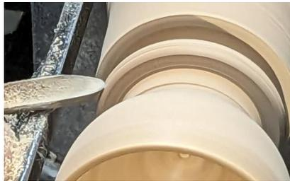
With a Bowl Gouge, David began the shaping of the first ring. The exterior of the ring needs to be done before separating the ring to float.
