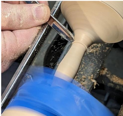
In order to complete the turning without rings in the way tape was used to trap them against the bottom of the cup part of the goblet. When the base part is completed, the rings are then moved to the base and the outside bottom of the cup is completed.
