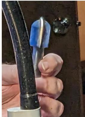
Sharing one of his "tricks of the trade" David used a router bit to make the initial hole in the end of the blank. This would become the interior of the cup part of the goblet and give a nice center to turn to inside, alleviating a problem often encountered when turning something like this. The router bit was mounted in a chuck in the tailstock in order to "drill" into the end of the blank.
