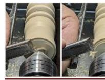
Skew chisels can also be used to square and flatten the end of a spindle as shown at the left.
