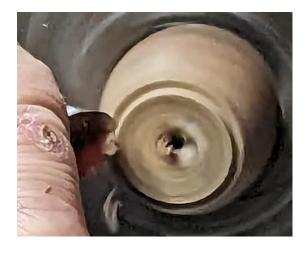
Once faced off, a small area is shaped to begin the location of the threading operation.
