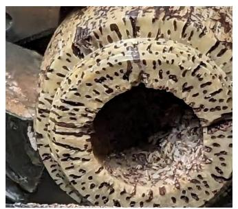
Voila! The threads are complete, the interior is hollow and not it is time to finish turn the exterior of the "acorn".
