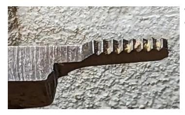
This tool will produce the internal threads on the cap which is still to be turned.
