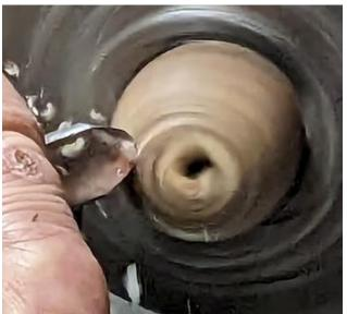
Using a small spindle gouge, Anthony begins to turn the shape of the nut to the finished size. The hole will become a hollow inside the turning and allow the "hiding" of small articles inside.
