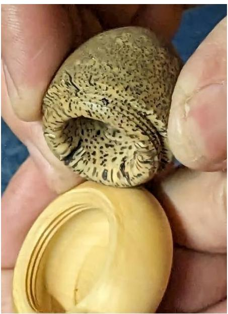
The completed assembly is shown at left with the "cap" having been disassembled from the "body" with matching threads interior and exterior.
