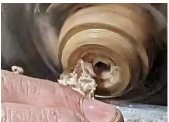
Once threaded, the interior is hollowed out. It is "safer" to leave the interior solid during the threading to allow more "backup" for the threaded part. Surprisingly, the nut composition is dense and even though what appears as a flaw, it is hard and solid.
