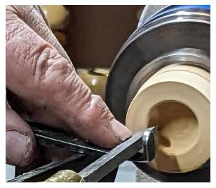
A special purpose tool is used to hold the threading tool in the photo at right. This allows a much steadier positioning of the threading tool and makes the threading process much easier than just using a tool rest alone.
