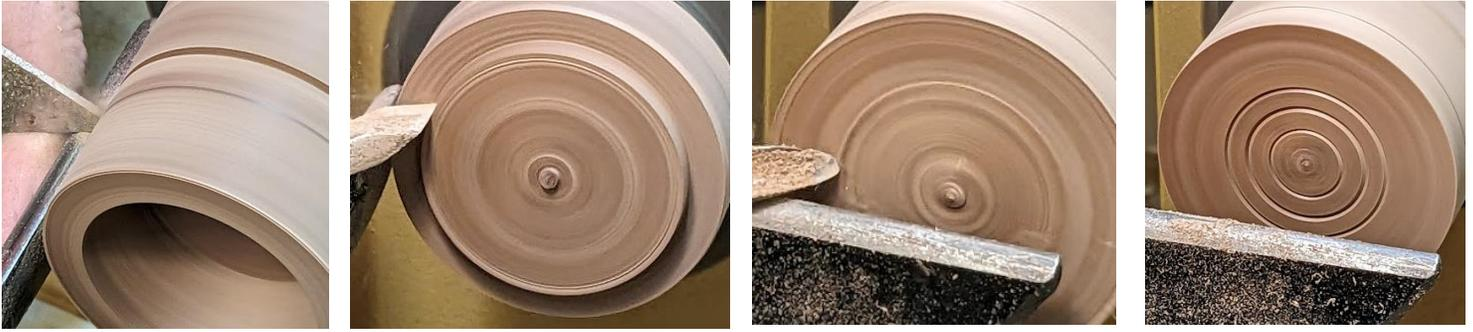
Upon removing the box body with the thin parting tool, the flange needed to be shaped to fit into the box. Last step in making the box was to decorate the bottom of the piece as seen at the far right.
