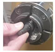
One more example of a screw center used on bowl blanks by drilling a hole, screwing the blank onto the screw up flush to the chuck jaws and then proceed to turn the blank. The hole goes away when the bowl is hollowed.
