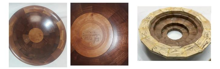
**Steve Dougherty** brought a segmented bowl (plate?) that he made from **Walnut** and **Cherry**. At the right is the process of assembling the parts before being turned. Note the hole in the middle. This was filled with the **Cherry** insert as seen in the middle picture above. Finished with a satin lacquer it really looks nice. Nice job Steve.
