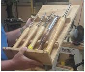
The next is a lathe tool holder that sits on the lathe to prevent tools in use from: a.) falling on his foot,
