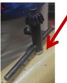
This handy little add-on is a magnetic button on the back of his chuck key. When using the Drill chuck this allows the key to be available without getting mixed into the chips, falling on the floor or some other annoying happenstance.
