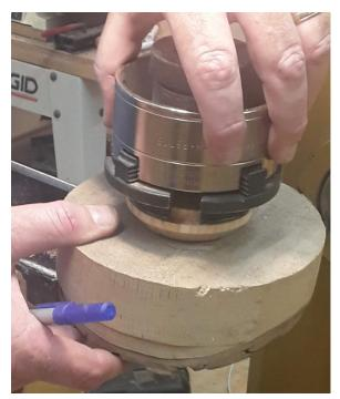
David prepares to mount the chuck with a backup piece of wood to allow some hollowing before removing from the chuck
