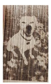
Here is what a scanned picture comes out looking like using the laser machine. This piece of wood is about  $3-1/2 \times 5-1/2$  birch. Closed grain wood will give a better representation of the image being burned onto the wood. Open grain detracts from the details and may or may not give a sharp laser engraving.
