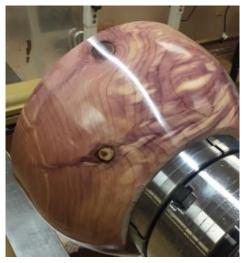
The FRICTION POLISH gives a more protected coat than the sanding sealer and looks deeper and slightly shinier that the sanding sealer.
