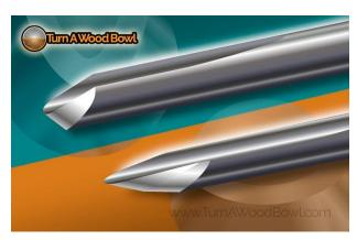
The bowl gouge flute is curved with wings and designed for turning wood bowls. A spindle gouge has a more open flat flute and is best used for details and spindle turnings.
