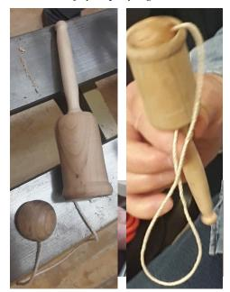
Danny's first step was to use a 2" square Maple blank about 4" long to make the "cup". After turning a small spot in the center of the blank Danny proceeded to turn the shape and make a hole for the cup part. Next he changed the tailstock to a large tapered center attachment to go into the cup and inserted a block into the chuck. With a stub to go into the handle hole in the cup blank, he mounted the rough turned cup onto the stub and brought the tailstock onto the cup hole.
