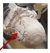
Beginning with a square spalted piece this is the result. Note above where the RED arrow points. A chip flew off but continuing to turn the ball part, a much smaller diameter is needed so ...
