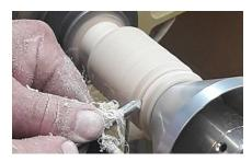
After turning the cup part round and sanding the outside, this is the "finished" cup at right. The part sitting on the lathe ways has a hole to be used for inserting the handle after it is turned. (see below)
