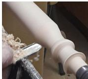
Note the piece by the tailstock. That becomes the part of the handle that will go into the bottom of the "cup" part. After turning the handle shape, a little sanding and the handle is ready to be checked as to fit.
