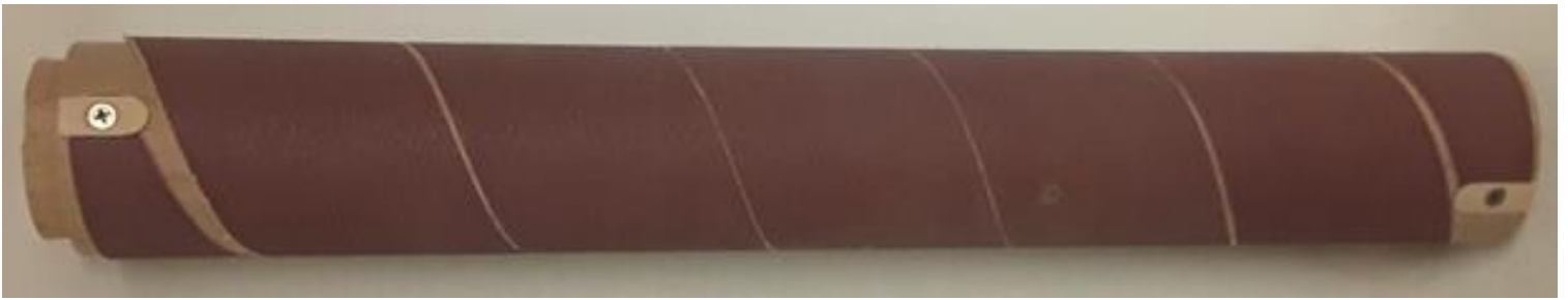
This is another view of Carl's sanding drum. Note the paper anchors on each end.
