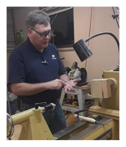
Now for the "Two-fer" demo. Chip Siskey showed the process for making a backing block or how to turn a blank without putting an inset to mount in a chuck.
