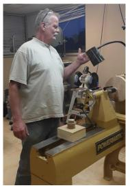
The feature for September was a plate turning by VP Danny Smith. Beginning with a slab of Maple about 2" thick Danny first trued it in the lathe between centers. This was after approximating the center on each side. The next step was to true the side away from the headstock and turn a slight taper to this side. Note the progression below.
