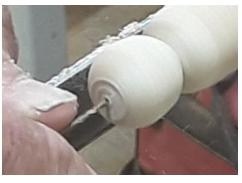
With the parting tool shown at left on top, Danny removed the first ball, drilled a small hole in the end of the second ball and proceeded to remove the second ball.
