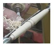
The final step required turning a taper on each half to give the spindle its final shape. Both ends are shaped alike to give a symmetrical look to the spindle. After light sanding the spindle, marks were made on either side of the bead in the center. Using the tool made as Project 1 for the evening's demo, Danny proceeded to burn in decorations on either side of the bead. Again light sanding to remove burrs left by the decorating completed the spindle.
