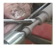
Shaping the second part and beginning on the third part of the finial is shown below. Once that is formed, the fourth part is done. This makes for a delicate and VERY small turning at the top. Final touch-up of the bottoms of each section is then done and very light sanding is done to prepare for removal from the blank held in the chuck.
