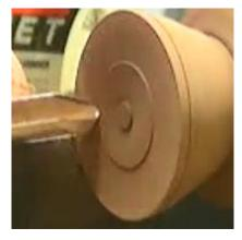
Next David proceeded to face off the end in preparation to establishing the interlock for the two egg halves. Note the initial position of the bowl gouge compared to the final position facing off the end.
