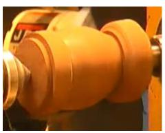
The progression from round to rough egg shape is shown above. The largest diameter is approximately in the "center" of the egg.
