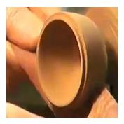
Final shaping of the top of the egg can be seen in the pictures above along with some finish sanding of the outside surface. Now all that remains is to release the egg half from the "pud" in the chuck.
