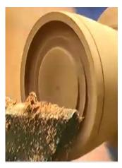
Changing from a parting tool to a beading/parting tool David began to establish the interior hollow of the egg part.
