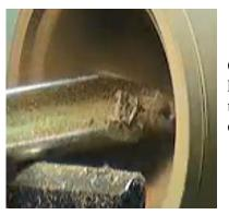
Continuing with the gouge, he hollowed and removed the nib in the center of the egg half.
