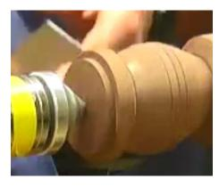
Using a narrow parting tool, David then proceeded to separate the two halves of the egg.
