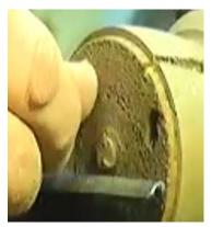
Upon removal of the finished half, the work remaining was exposed. Using his thumb, David indicated the rim needed to be left for the two halves to reassemble and stay put.
