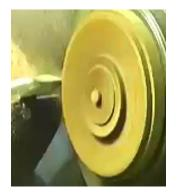
From removal of the "finished" turning a "pud" remains in the chuck. Using this, a jam chuck to hold the just-removed turning can be held to smooth where it was removed.
