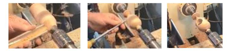
The main body begins to take shape on each end, first with a roughing gouge then with a small spindle gouge.
