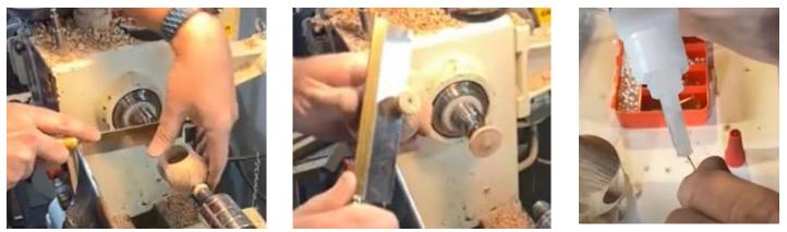
Rather than risk an accidental drop, a fine tooth saw was used to separate the turning from each end. The hanger was a gold plated fish hook with the hook removed into a small hole that had been pre-drilled before beginning the turning. A small amount of cyanoacrylic glue holds the hanger in the end.
