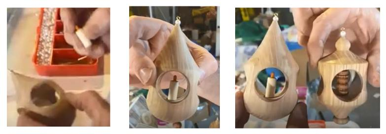
A small candle is inserted in the center of the ornament. Just a simple dowel rod turned and painted makes a great candle. At right is the comparison of the sample and the just turned ornament. It COULD be left natural and unfinished or it could be stained and finished.
