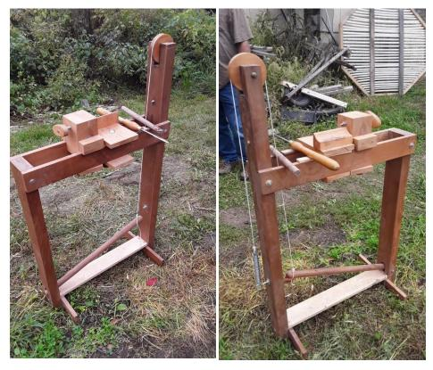
Another of **Danny Smith**'s finds/builds is this foot-powered lathe. Shown in the far left picture is the back side and in the near side is the operator side. At the lower left in the near photo is a spring that causes the rope to retract when pressure is released on the treadle at the bottom. Not sure how the turning is made to turn but I think it has something to do with wrapping the rope around the piece being turned(?).
