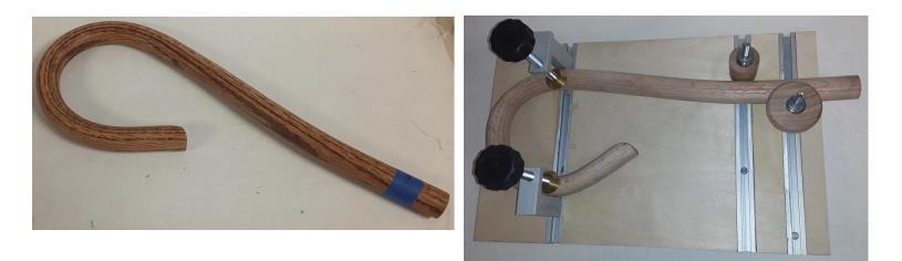
Club Treasurer **Chip Sisky** brought a fixture he uses to produce the crook at the top of the staff he produces for Bishops worldwide. The fixture is adjustable for several reasons: **a.** to allow insertion of the softened staff crook and **b.** to provide for any variations in design of the crook based on dimeter of the stock. On VERY close examination of the crook Chip brought, a small crack can be seen on top of the crook.
