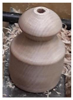
Light sanding at the part-off spot gives a biscuit cutter ready for a food-safe finish and –Voila! Ready for biscuit dough with the pusher in place.
