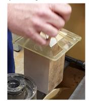
Next, a center finder was used to locate where to put the centers on the lathe.
