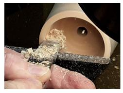
Progression from removal of the "pusher to layout of the cutter to interior shaping progresses. Since the biscuit size will be 2" the inside must be turned to approximately that size. Depth must allow for the pusher as well as the maximum thickness of biscuit dough—about ¾".
