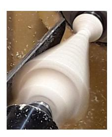
Shown below is the progression on the first "off-center" location. These slits will be colored on the finished turning. Note that only every fourth line has been turned so far. Each successive center will locate another set of slits one-third of the way around the "tree." Depending on which way the off-centers are chosen will determine the progression around the tree as one goes up the turning.
