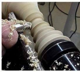
Using a special tapered tailstock, Harlan then finish turned the rest of the bell shape on top and parted it off.
