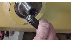
Using what normally would be a tailstock center, it was put into the headstock as a center. This allowed the workpiece to be held and yet slip between centers should too much pressure be used.
