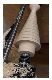
Once the shape progressed, lines were marked at regular intervals. These lines would become the spots where the offset turning would be done. Slits would become design elements in what would be a small tree-shaped ornament.
