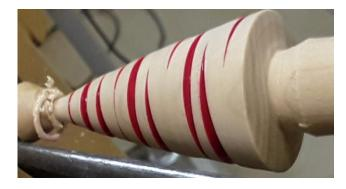
After slitting each of the three off-centers, coloring the slits with a permanent color, and turning the final smoothness, the tree is ready for finish turning.
