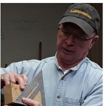
The first step was to locate the "ball" position on the wood blank. This is necessary to help keep the board turning true by placing both centers equidistant on the blank.
