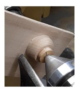
This is the result before separating the "ball" shape from the board. The ball doesn't actually separate in the sense that it is removable; only that it can turn inside the board location.
