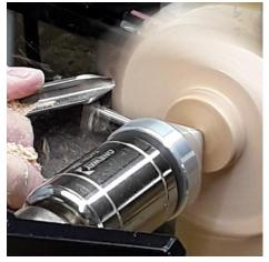
As turning commenced, the obvious "air" turning began. From a thick board came one that was much thinner with a "knob" on both sides where the "ball" would develop.
