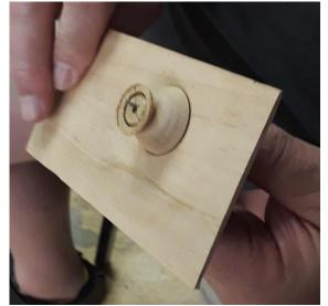
The semi-finished turning is now ready for hand work to complete the ball shape on each side of the board.
