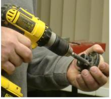
First, two temporary spacer chucks ends needed to be fastened to the mandrel. These chucks would go into the ends of the peppermill blank after a hole had been bored for the exit of pepper from the mill.
