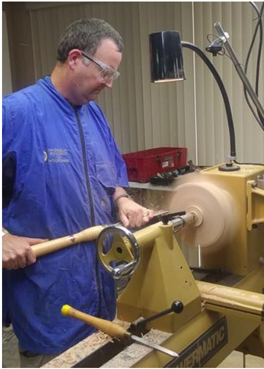
At left David is turning the lower face of the wing bowl and on the right the blank is being smoothed next to the headstock. Again David pointed out the importance of knowing where hands and arms are as the corners spin by.
