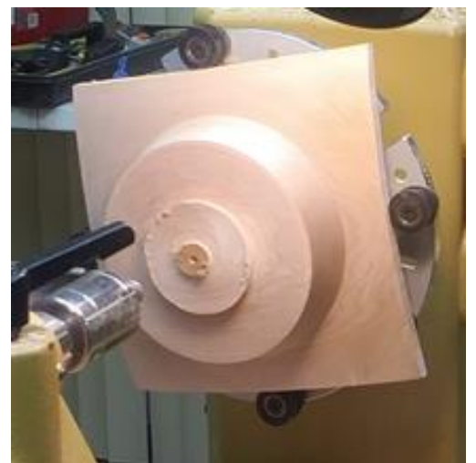
The bowl is now ready to have the final shaping on the underside. The points of the "wings" are still a hazard if hands get in the way, though.
