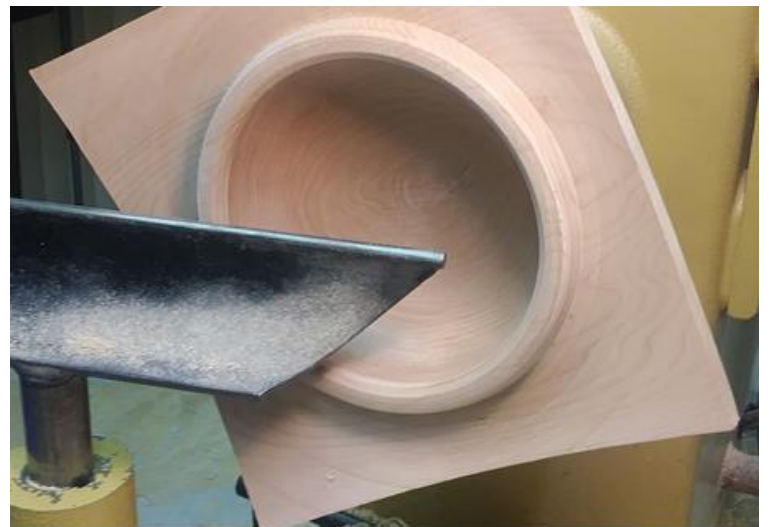
At left above is the back side of the bowl showing the curvature and general shape before thinning the "wings". At the right shows the inside of the bowl on the tailstock side with the depth and rim taking shape.
