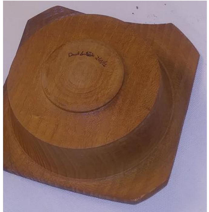
David Bartlett, program “celebrity”, brought two samples of his demo work. This is a wing bowl made from sycamore. The other sample is from what appears to be mulberry. The bottom area is slightly concave to allow for the tenon used to turn the piece.
