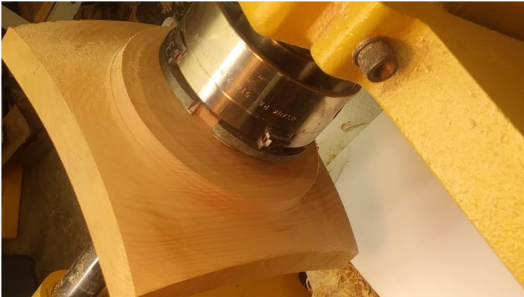
At left above is the back side of the bowl showing the curvature and general shape before thinning the "wings". At the right shows the inside of the bowl on the tailstock side with the depth and rim taking shape.
