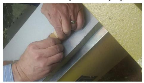
Shown here is the process of using regular yellow Titebond<sup>TM</sup> glue to fasten the segments together. If the cutting process is accurate two halves can be assembled and then fastened together. Once these have cured overnight they can be turned in a similar fashion to what was demonstrated.
