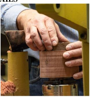
Once glued on with CA glue and set, the turning begins. Inside details are turned to size first and checked before beginning the outside shape.
