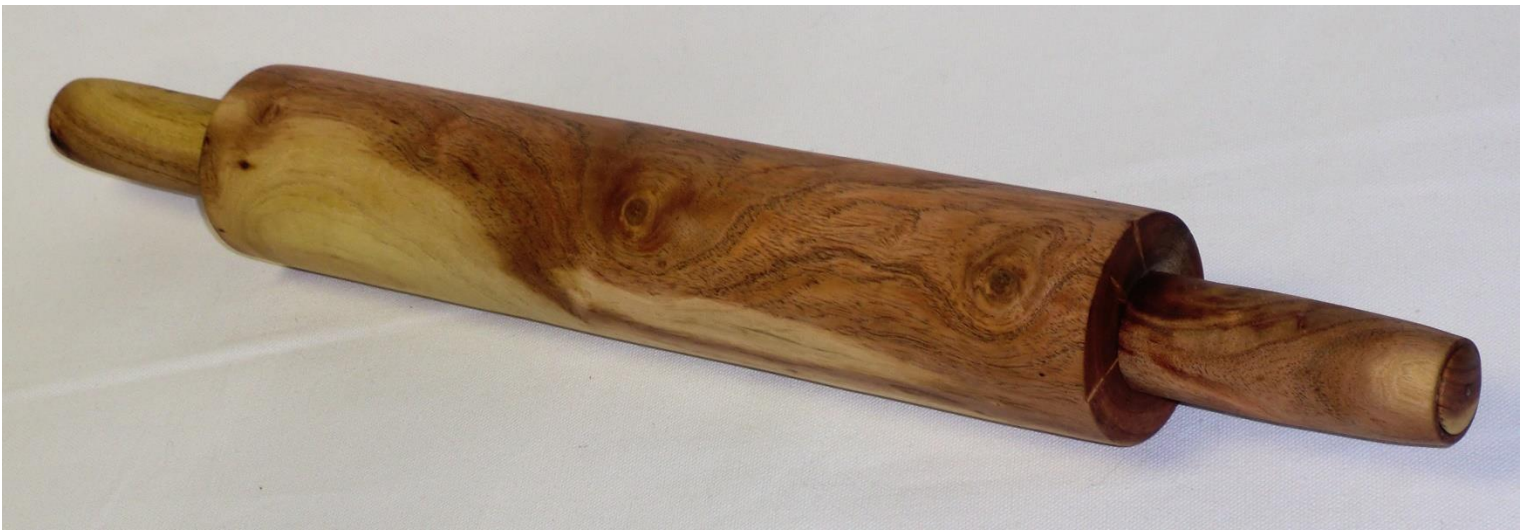
Kent Townsend-- Rolling pin made from Mesquite. Diameter of main body is about 2-1/2" in diameter and about 12" long with 3" handles on each end. Handles are about 1-1/4" in diameter to accommodate someone with arthritis in their hands. Finish is several coats of flax oil.
