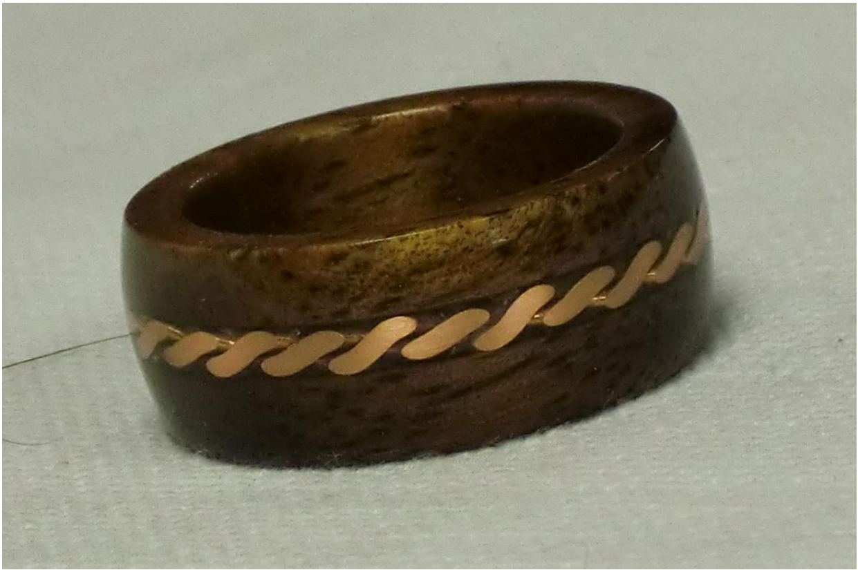
Mikeal Jones- Ring made of Mahogany and twisted Copper wire embedded in CA glue. Groove at the bottom of the embedding is flat-bottomed to allow the wire to lay evenly. Size is about a #9 ring size. (enlarged here to show detail)
