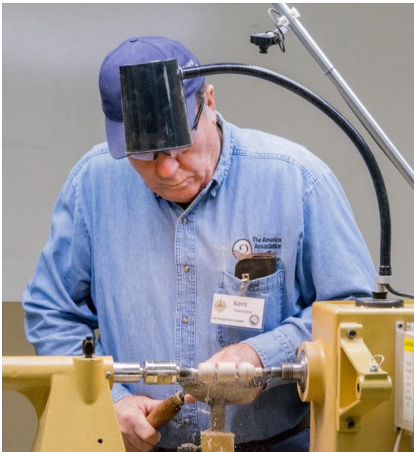
Kent Townsend begins a baby rattle. The wood is hard maple and is about 1-1/2" square by about 8" long as a blank. After laying out the basic shapes and turning the two end pieces into round balls, the center is ready to make the two rattles. Note in the following pictures on page 5 the progression from bead to rattle pieces.
