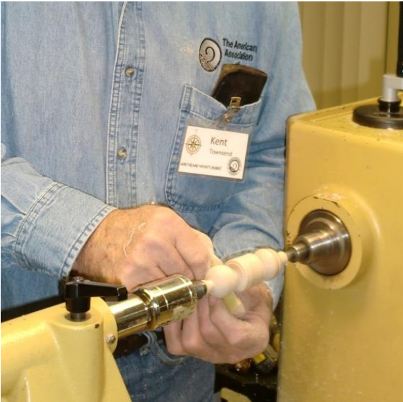
Kent Townsend begins a baby rattle. The wood is hard maple and is about 1-1/2" square by about 8" long as a blank. After laying out the basic shapes and turning the two end pieces into round balls, the center is ready to make the two rattles. Note in the following pictures on page 5 the progression from bead to rattle pieces.
