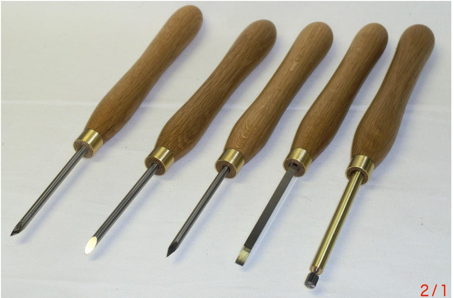
Andy Brundage-- Turning tool set. These tools are made from tool steel, both round and square. The tool on the far right has a special insert with pressed-in bearings so the insert can turn. Body is made from brass tubing. Handles are turned from oak with brass ferrules.
