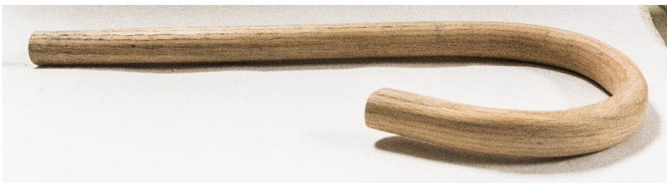
Steam- bent Bishop's Closier by Chip Siskey
